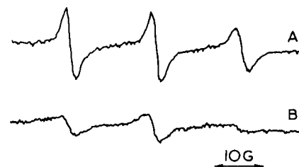
Figure 2 E.s.r. line shape change upon duplex formation between (RUGT, U) n and (A) n in 0.195 M NaCl, 0.01 M Tris, pH 7.5. A, 2.9 × 10 -5 M (RUGT, U) n ; B, 2.9 × 10 -5 M (RUGT, U) n ·(A) n
